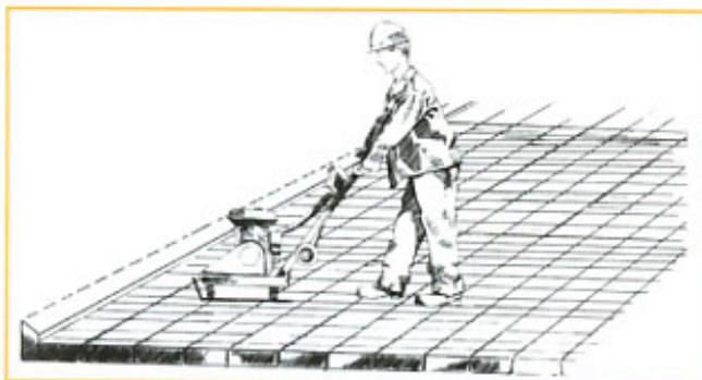
Figure 19: Vibrating the jointing sand into the joints
