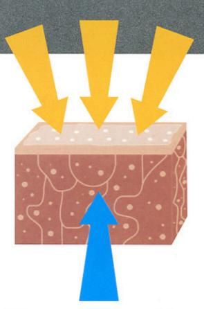
Efflorescence emerged from pores within a magnified area of a concrete paver.
